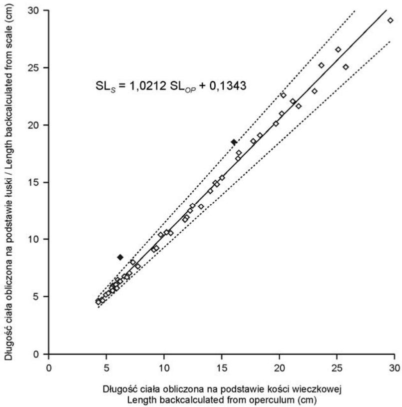
Figure 23. Relationship between lengths at age back-calculated from scale ( $SL_S$ ) and opercular bone ( $SL_{OP}$ ) of the same individual. Solid diamonds indicate points out of the 10%-range of the average estimate of  $SL_S$  from  $SL_{OP}$  (the range is limited by dotted lines).
