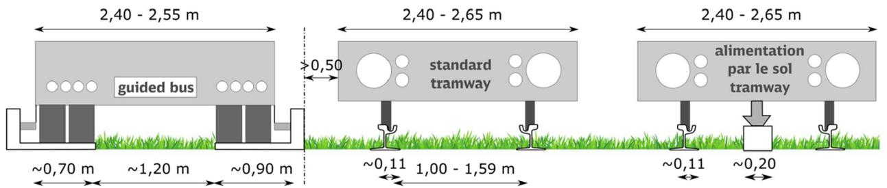
Figure 5. Space for greenery in tracks of guided buses, typical tramways and tramways supplied with electric power by the conductor rail built into the track (*l'alimentation électrique par le sol*).
