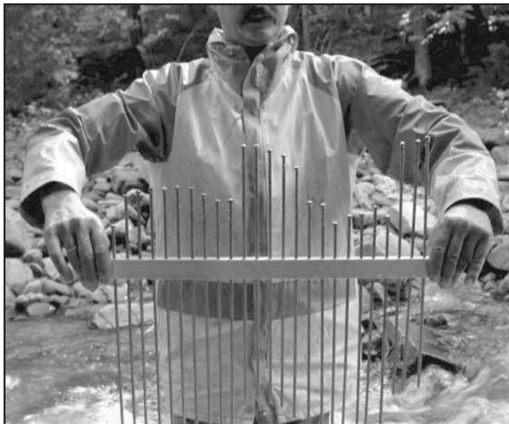
Fig. 3. The stream bottom roughness measurement device (see methods for explanation).
